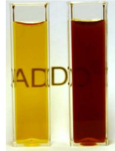
Motor oil with ADDO (left) and without ADDO (right) after 25000 km run.
